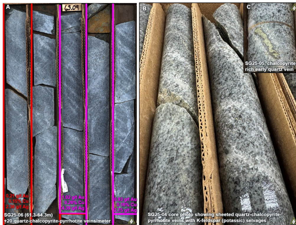
Figure 10: Core photos from SG25-04, 05, and 06 highlighting key porphyry mineralization styles and associated grades with sheeted to stockwork quartz-pyrrhotite-chalcopyrite veins cutting Jurassic quartz monzonite.
