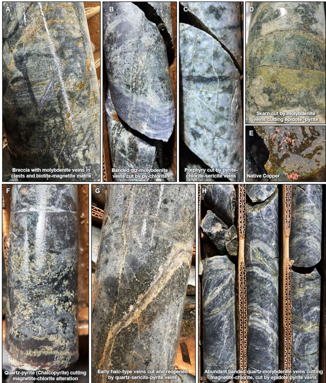
Figure 5: Select core photos of representative porphyry vein styles and mineralization – clear evidence of a porphyry system at the Climax target and proximal to a potential copper center.
